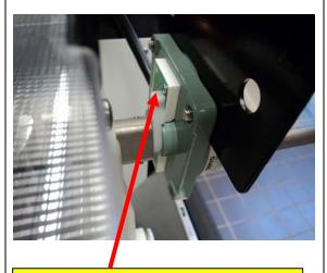
Hall IC Switch is located on the motor backside. (Magnetic Switch)
